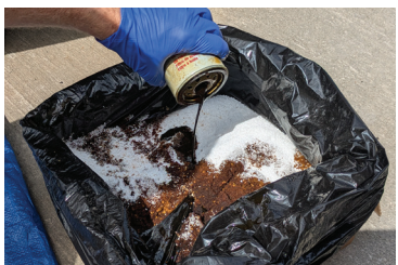
DRAIN FILTER OIL & PLACE INTO AGGREGATE
